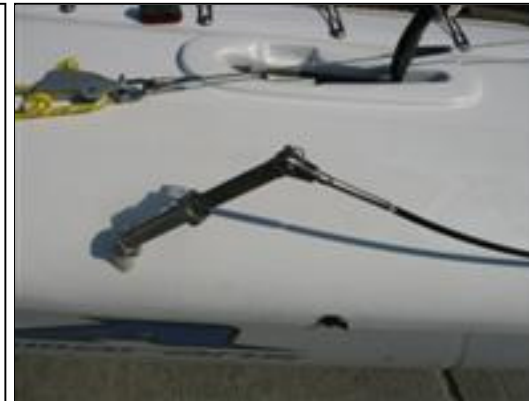
Fixing the stays and trapeze wires Step 1 Maximize staymaster/stay adjuster length
