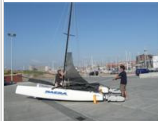
Step 3 Make sure the mast and the sail are facing the same direction while locking!
