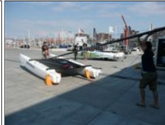
Step 3 Put your foot on the mast base to prevent the mast from coming off the ball!
