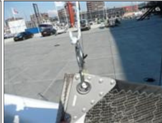
Raising the mainsail Step 1 The knot should face the mast
