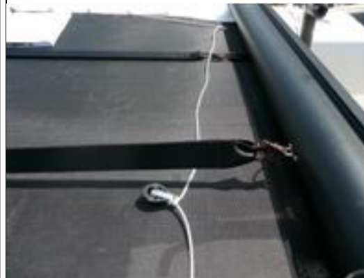
Spinnaker retrieve block Step 1 Go under all the foot straps!
