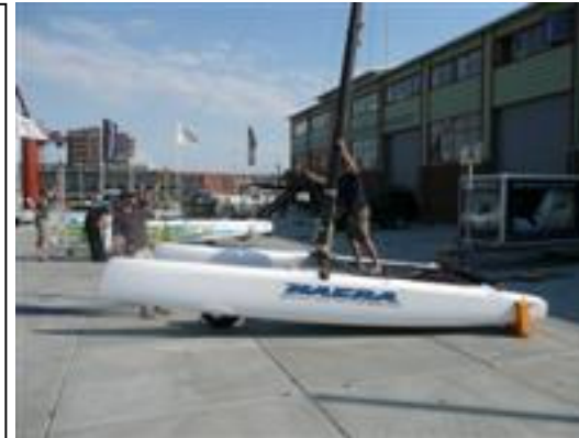
Lowering the mast
