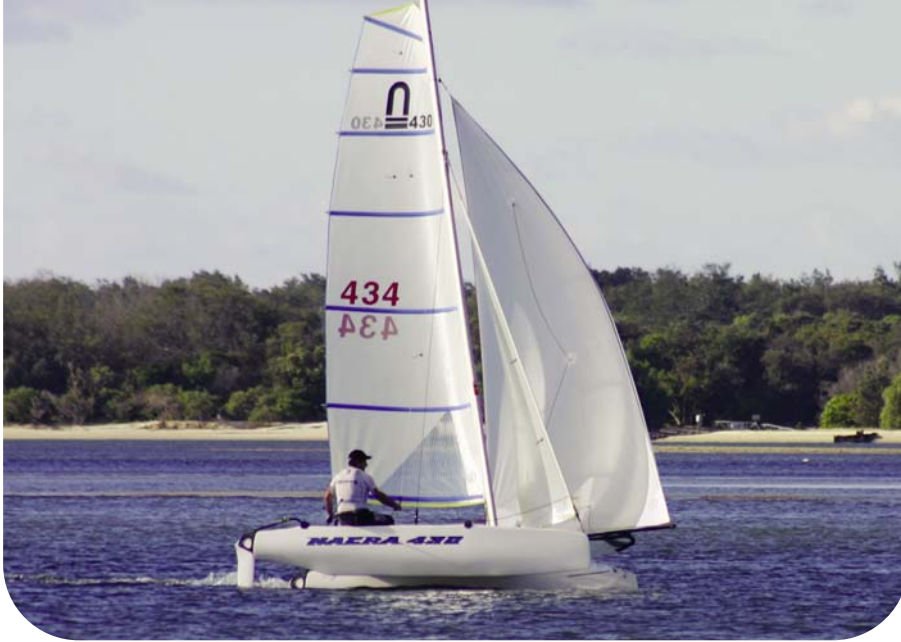
Nacra 430 Rocket – showing the large volume hulls which were made to take extra loads of using a spinnaker.
